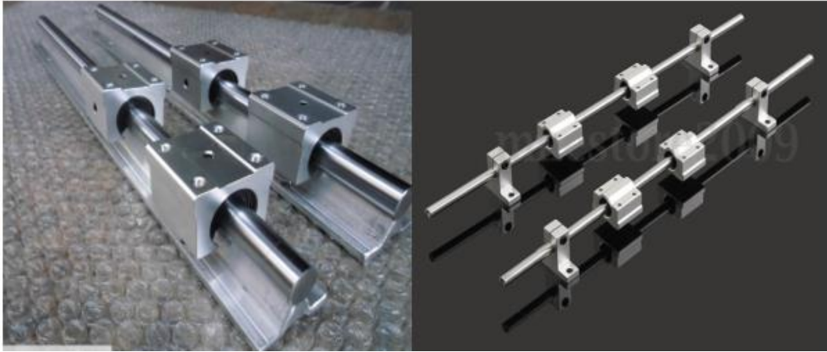
Figure 12: Linear rail systems with open bearings on the left and closed bearing on the right [17] [18]
